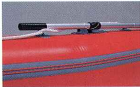
RUBBING STRAKE provides extra protection from contact with docks and other objects.
