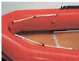
INTERIOR SAFETY LINE extra passenger safety.
