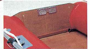
WOOD TRANSOM is protected by aluminum motor plate.
