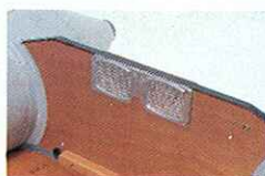
PROTECTIVE MOTOR PLATE protects the wood transom from motor clamps.
