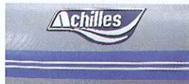
FULL-LENGTH RUBBING STRAKE for extra protection in collisions with docks and other boats.
