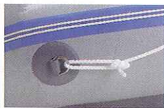
TOWING BRIDLE to make it easy to tow in the best possible manner.
