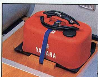
FUEL TANK PAD
