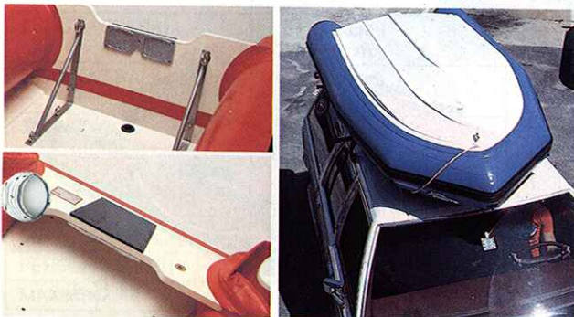
The fiberglass transoms of HB boats fold down for easier transporting and storage than other rigid hull inflatables. The modified "V" hull design makes HB boats faster.
