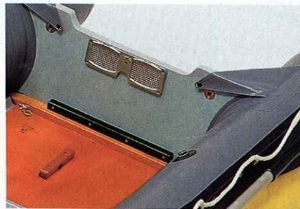
Fiberglass transom and aluminum motor pad.
