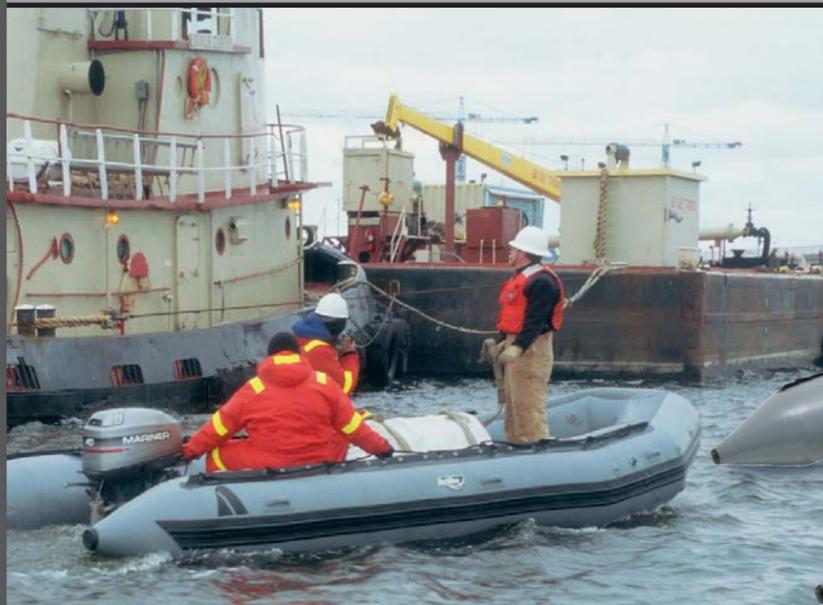
**SU boats** feature an additional heavy-duty layer of 840 denier nylon fabric in a two-ply technique that results in a core fabric even stronger than a single base fabric of equal thickness. This tough, durable fabric, along with a host of special commercial features such as recessed valves and a full-boat, reinforced cargo/step patch, make these the most rugged multi-use work and utility boats around.
