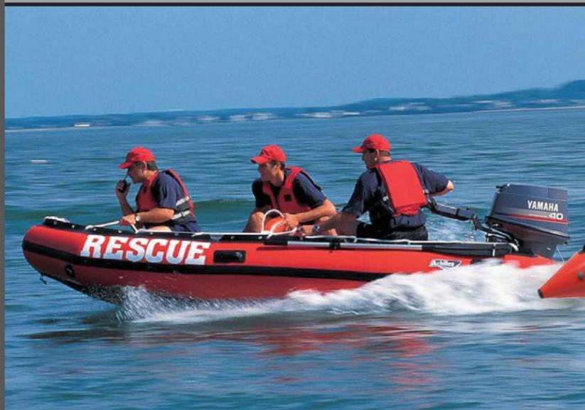
**These rugged models** offer both the room and performance to fill a range of needs. Their size allows them to carry a fully equipped team of divers or rescue personnel for any situation. Their tough Hypalon® fabric and aluminum floor systems stand up to all types of heavy use. A deep "V" trigon air keel insures better tracking and performance when speed is of the essence.
