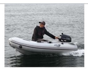
We've incorporated all the best features of our pacesetting HB fiberglass hull inflatable boats into the HB-AL series. These rugged boats feature a marine grade aluminum hull that is powder-coated to ensure a smooth, long lasting finish. They offer the advantage of being lightweight yet remarkably strong and durable. A modified V hull, combined with their lightweight allow HB-AL boats to cut through water efficiently with less horsepower.
