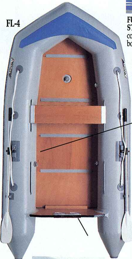
PROTECTIVE MOTOR PLATE protects the wood transom from motor clamps.
