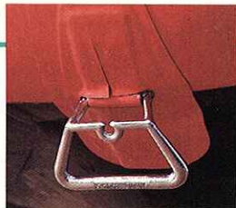
A heavy duty stainless steel bow carry handle is standard on Achilles sportboats
