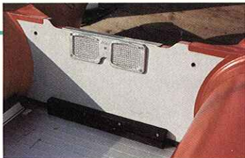
Fiberglass transoms with motor pads are featured on most Achilles sportboats.
