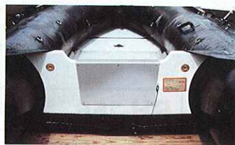
Extra tough aluminum plate to protect transom from outboard motor.
