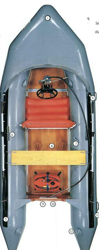
Bilge Drain: Self-bailing drain with rubber diaphragm check valve.
