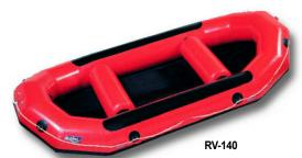
Nothing has been left out in making Achilles RV Series riverboats the strongest available for professional use. Both the 840 denier tube fabric and the additional 840 denier fully-wrapped floors are coated with DuPont Hypalon® for unsurpassed protection against damage from abrasions, punctures and weathering. All "D" rings have been strengthened to last on all
