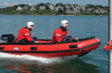
**FRB boats** are designed to enable fire departments and emergency rescue units to keep an easily stored boat available that can be ready in minutes to respond to a water emergency. Remarkably light weight, they are easy to carry, yet can hold up to 1230 and 1500 pounds respectively. They inflate quickly using compressed air bottles or the foot pump included as standard equipment.
