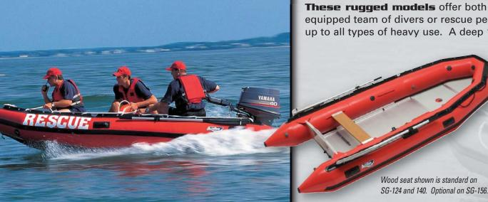
**These rugged models** offer both the room and performance to fill a range of needs. Their size allows them to carry a fully equipped team of divers or rescue personnel for any situation. Their tough Hypalon® fabric and aluminum floor systems stand up to all types of heavy use. A deep "V" trigon air keel insures better tracking and performance when speed is of the essence.
